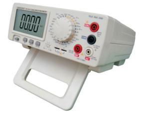
Overload protection in all ranges. Its Input Impedance is 10MW. AC measurement is performed by high accuracy
