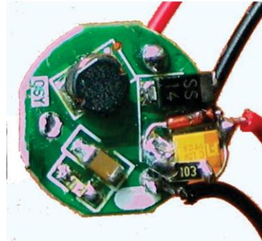
This means you cannot put a milliammeter (this is the correct wording for a milli-amp meter) in the positive line and expect the circuit to work correctly. The high-resistance of the meter will cause the output to decrease considerably. To get around this, a 1 ohm resistor (brown-black-gold-gold) is placed on the positive rail and a multimeter (200mV or 2v range) is connected across the resistor. This means each mV reading will represent 1 mA current.
