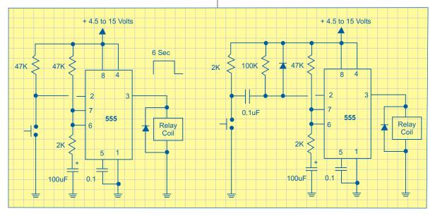
555 timer circuits are used to time and control the intermittent operation of circuits and equipment (time ON vs. time OFF).
