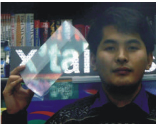
Fig .10. An optical Camouflage Application using RPT
