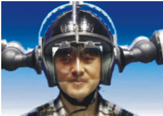
Fig .9. Head Mounted Projector (HMP) with RPT
