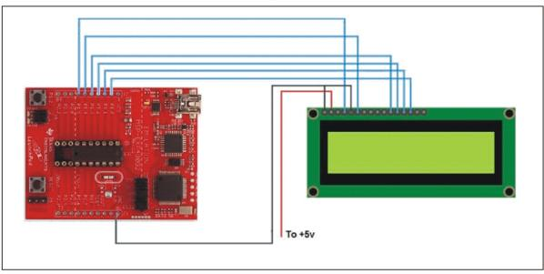
Additionally, every pin of the MSP430G2xx device is fully accessible, allowing easy interfacing of external components or custom daughter cards. Since the launchpad works at 3.6v, we need to provide an external 5v supply to power the LCD module. But we can directly connect the port bits of MSP430 to LCD.
