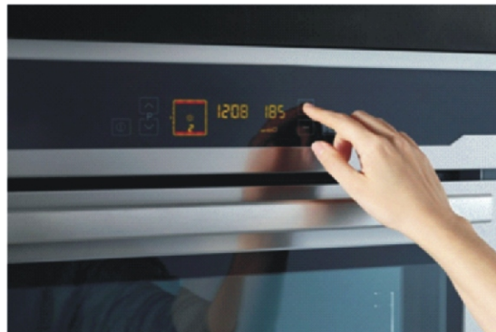
Fig. 1 (b): Touch-sense based user interface
