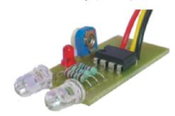
distinctive manner. Sensors used in the robots works in the same way as the eyes in the human being. The sensors used are IR sensors. It emits and detects IR.
