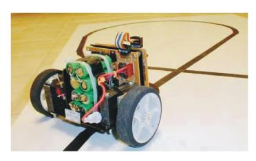
i.e. they emit the light in a straight line . So ,by using this property , we used them as the communication network . For detecting , we use three detector in each of the two other robot . These detectors are mounted in the middle of their front . They are uniformly spaced apart at a distance of 0.8 cm
