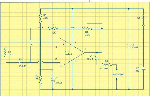
example, the electric field around a mains transformer can be heard as a 50 Hz hum. The POT R4 can be used to adjust the gain of the amplifier. By keeping the sensor inductor near to a telephone line, you can even hear the telephone conversations.
